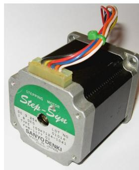
Figura 3. Motor STEP-SYN 103H7124-0740
